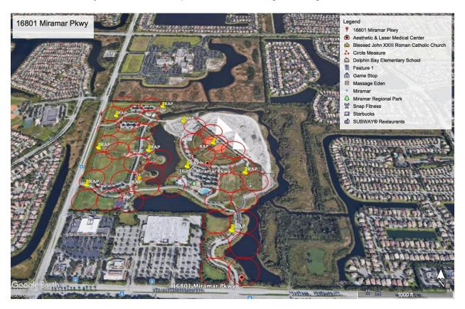
A pre-site survey was completed by Cisco, any Yellow pin is an approximate location that will need Fiber installed to and or another form of service delivery. Each Red circle is to be an access point. Mesh connections are assumed but by design should be limited to 1 hop.
